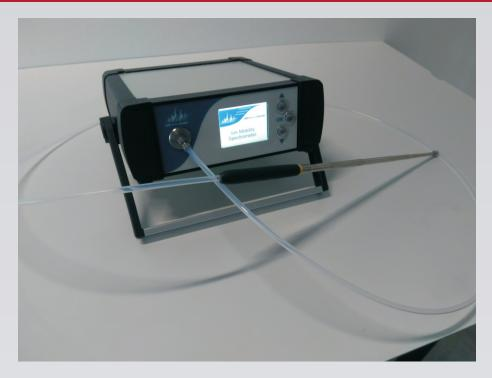
The **CWAe-Analyzer** is a multi-gas analyzer for the high-sensitive detection and identification of Chemical Warfare Agents (CWAs), Homemade Explosives (E) and/or Toxic Industrial Chemicals (TICs) without any enrichment directly on site already at a very low concentration level. They have been developed by IUT/IUT Medical over more than 20 years. It is best suitable for the use in homeland security, building protection, and general CBRN applications.
